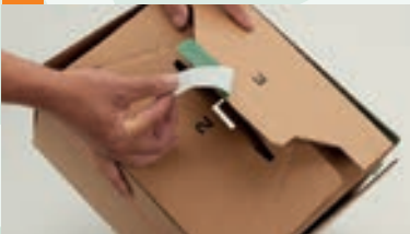
Stick the base flaps inward; stick the closing flaps using the progress self-adhesive seal
